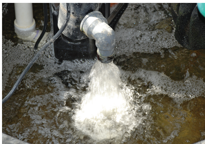
Figure 8. Submersible impeller pump with waterfall aeration.
