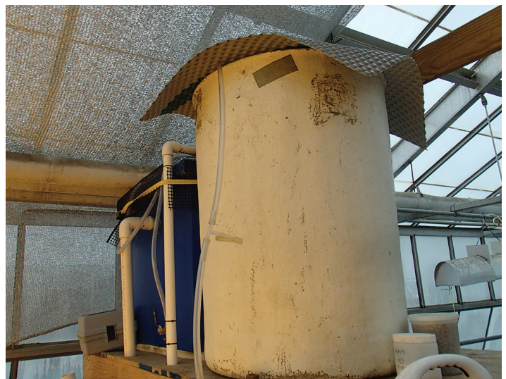
Figure 12. Head tank with covering to prevent algae.
