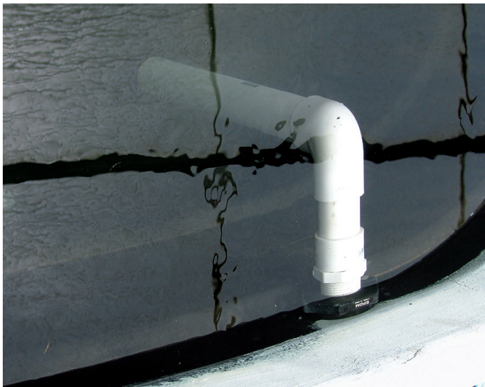
Figure 3. Solids lifting outflow.
